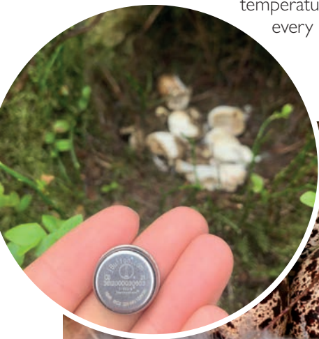
iButton thermocouples are placed in nests and used to measure nest temperature.
