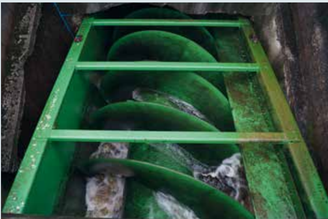
John's Archimedes' screw generates enough power for 90 homes
