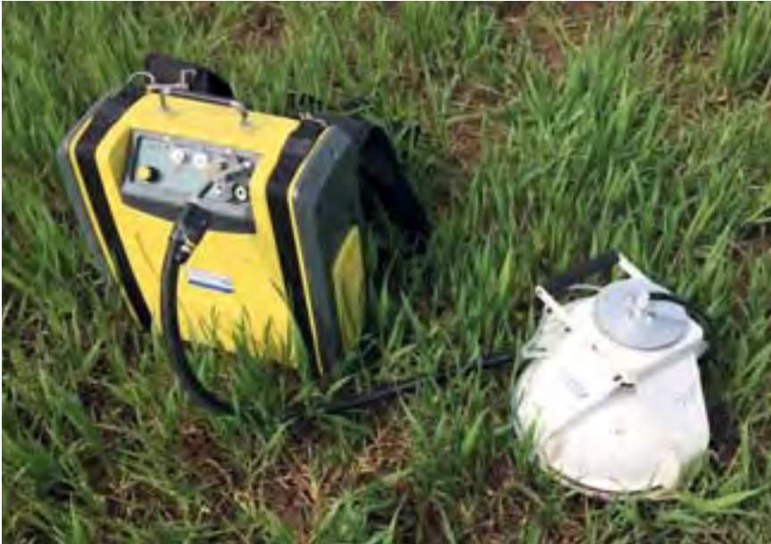
The Gaset GHG analyser monitors greenhouse gas flux in the crop. © Jenny Bussell/GWCT
